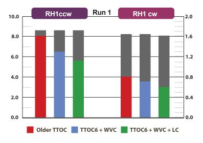
Similar results can be seen for the Radial Force First Harmonic (RH1) in the chart below. This data is from the same set of 5x5 certification tests. Again, the average measurement value is practically unchanged, and the measurement range is reduced significantly.
