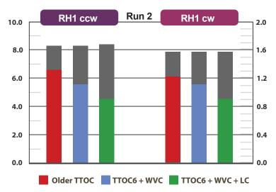
During certification testing, abnormally high values within a set of passes of the same tire are commonly referred to as 'outliers.' In all 10 sets of 5 tire passes, the TTOC6 software with WVC and LC algorithms reduced the highest RPP and RH1 measurements by an average of 0.21 lbs. and 0.25 lbs. respectively. Of these 'outliers,' 90% of the TTOC6 + WVC + LC measurements were lower or equal in magnitude compared to older TTOC measurements.
