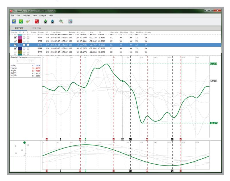
Overlay any or all splice values on a waveform or harmonic.
