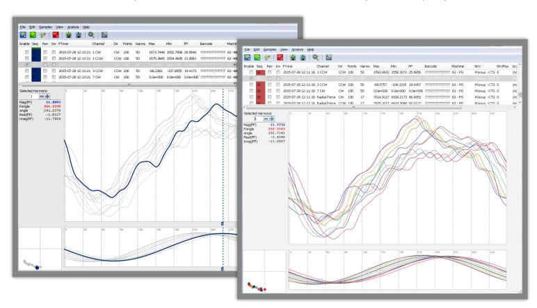
Plots for visualization of tire data include: Complex, Individual Harmonic, Waveform, Harmonic Magnitudes, and Trend.
