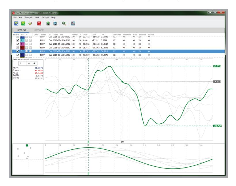
Once you import a set of tire waveforms, quickly view, analyze, and manipulate waveform data to see its effect on harmonics and peak to peak values.
